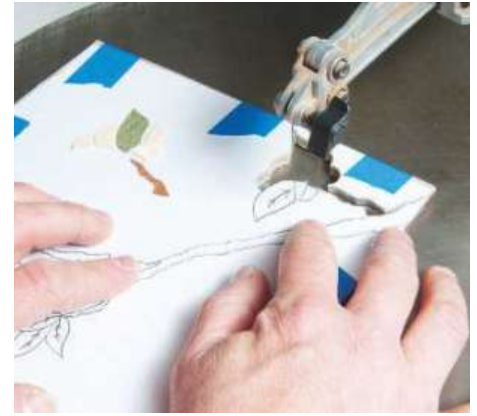
▲ Pic.3 Using a scroll saw fitted with a 2/0 blade on a low setting, start with the outside pieces and cut each part one at a time
